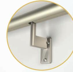
Patented twist-lock L-Brackets easily pivot for slopes and support over 225kgs each. Spacer Brackets included as required under the New Zealand Building Code.
